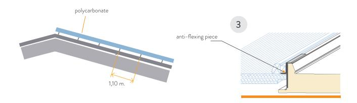
• **Drill** the sheets with holes at least 3 mm larger than the screw body. DO NOT SCREW DOWN with excessive pressure, to allow movement of the sheet when expanding. DO NOT install sheets with induced stresses that can render them brittle or cause microcracks (pict.4).
