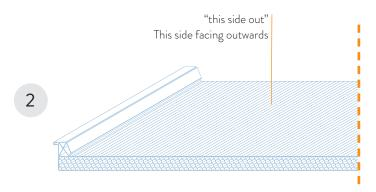
• We recommend that polycarbonate sheets be fitted with a maximum span lengths of 1.100 mm for roofing enclosures; for spans greater than this it is advisable to use anti-flexing parts (pict.3). Check with our technical department for the minimum cold bending radii of this material.
